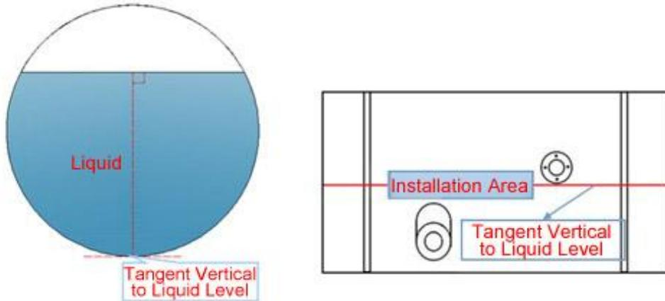
Figure 14: Installation Area of Round Fuel Tank
