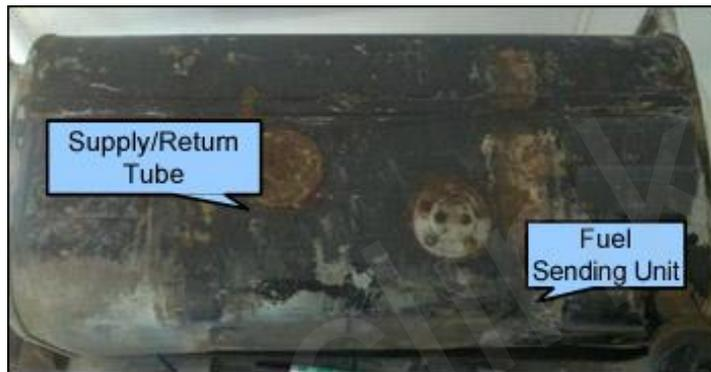
Figure 8: Surface of Square Fuel Tank
