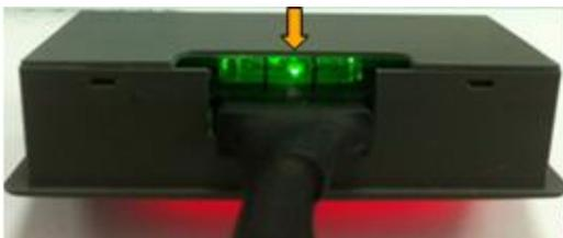
The green part is a level tester. If the bubble is in middle, it means the fuel tank is horizontally placed.
