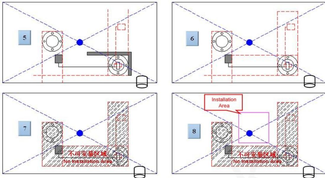
Figure 12: Locate the Installation Area
