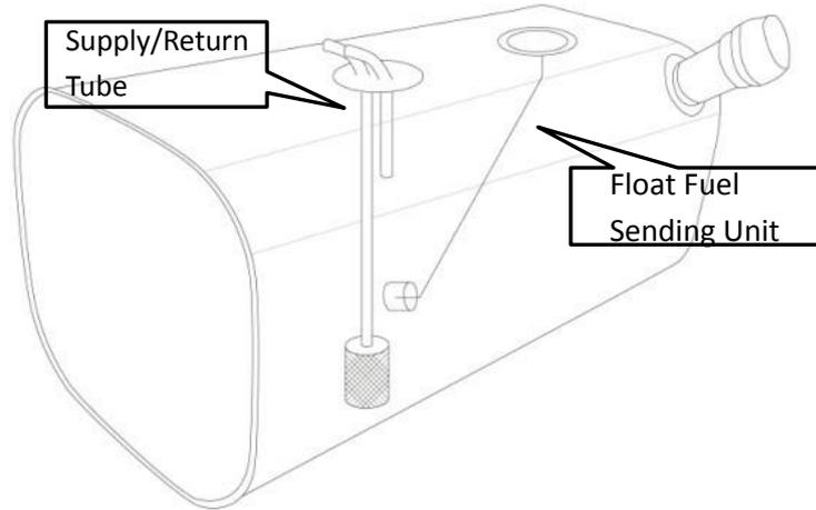
Figure 9: Locations and Structures of Obstacles in Square Fuel Tank
