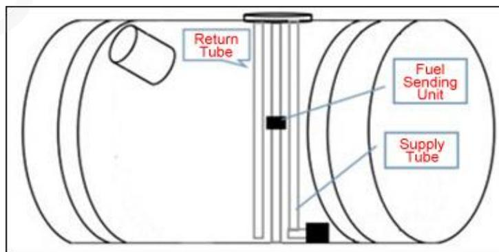
Figure 11: Locations and Structures of Obstacles in Round Fuel Tank
