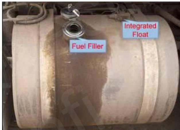
Figure 10: Surface of Round Fuel Tank
