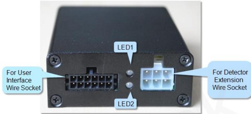
Figure 5: Signal Control Box Interface
